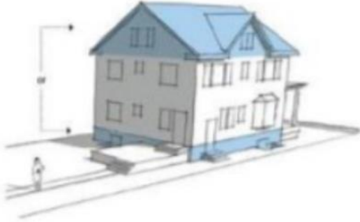
Interior ADU: Attic or Basement
