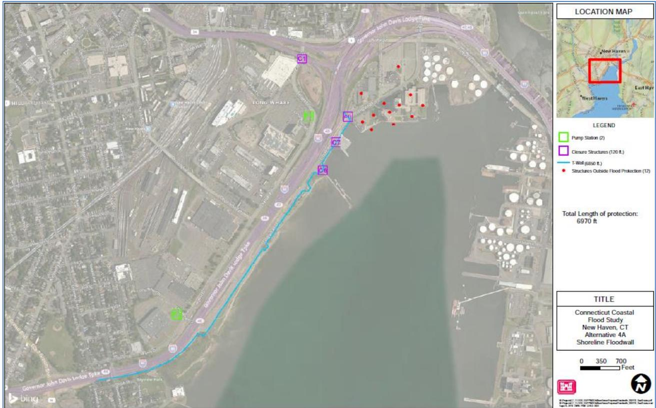
**Figure 13. Alternative 4A, (Shoreline Floodwall)**
