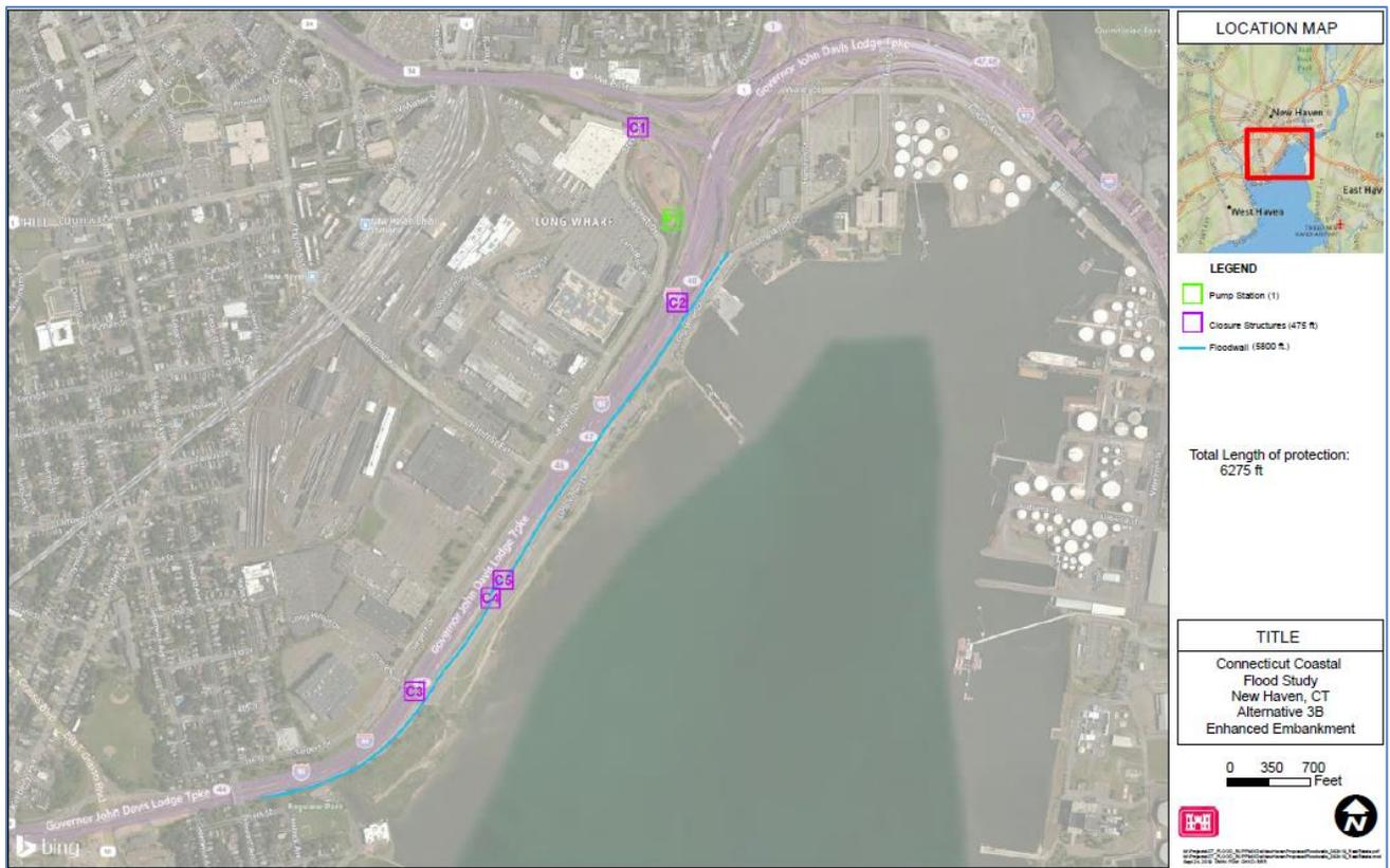
**Figure 12. Alternative 3B, (Enhanced I-95 Embankment)**
