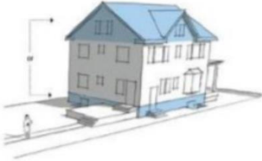
Interior ADU: Attic or Basement
