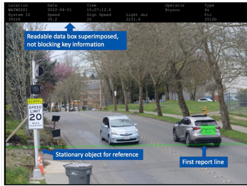
First Image in Color: Vehicle exceeding speed, showing first report line, configurable data box superimposed not blocking info
